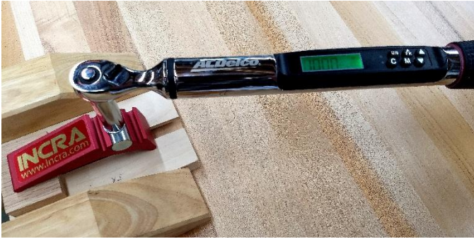
Applying instrumented drive torque to a test specimen
